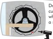
Drill through the curtain and drum wheel rim and fix with a self tapping screw.
