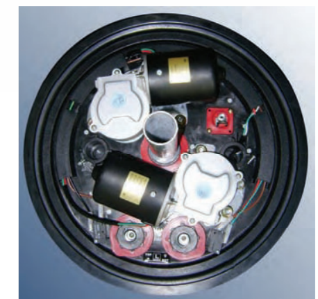
Front View of IGDU unit showing twin 24Volts DC Motors, Limit setting cams etc..
