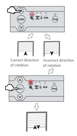
**3** Briefly press the PROG button until the door jogs to complete the motor set up procedure. The motor & safety brake LED goes out and the safety edge LED comes on.
