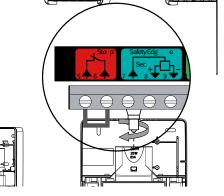
**2** Use the ink provided to connect terminals 5 & 6 if no safety brake is required.
