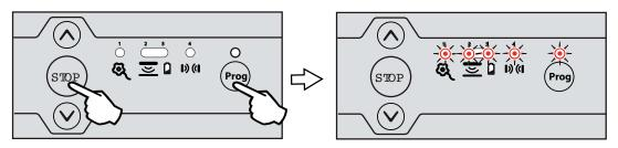
**2** Entry into programming mode by pressing button PROG the receiver is locked.
