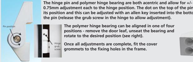
0.75mm adjustment each to the hinge position. The dot on the top of the pin shows its position and this can be adjusted with an allen key inserted into the bottom of the pin (release the grub screw in the hinge to allow adjustment). The polymer hinge bearing can be aligned in one of four
