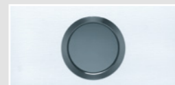
Porthole with stainless steel frame, with 10-mm double acrylic glazing** Dimensions: inside: approx. ø 290 mm outside: approx. ø 350 mm
