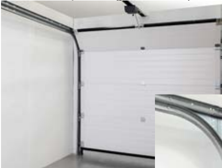
Side extension springs assist the lifting of the door on smooth-running rollers into the overhead tracks.
