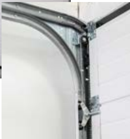
Side extension springs assist the lifting of the door on smooth-running rollers into the overhead tracks.
