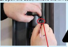
Do not attempt to remove the hinge cover without releasing the set screw. Damage will occur!
