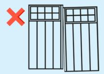
The top edges of each leaf should be horizontal and level with each other.
