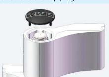
2. Open the door, remove the M4 screw (3mm allen key).
