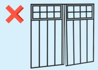
The door leaves also need to align vertically with the leading edges of each leaf aligned along their full length.
