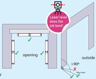
Openings must be plumb and square and the floor area within the arc swept by the door leaf must be level or fall away from the opening.
