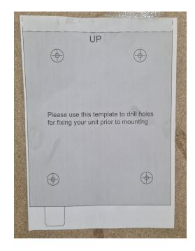
Using the "drill hole mounting template", mark hole positions desired.
