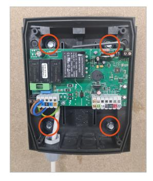
Use appropriate fixings to mount the panel to the structure in the highlighted locations.
