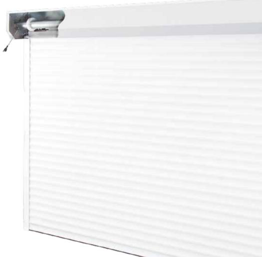
Gliderol Insulated Roller Doors take up very little space inside your garage. The standard configuration, using 77mm foam filled lath (Also available as a manually operated system), requires 300mm of headroom and is supplied with 70 or 90mm guides depending on specification. The compact version, using 55mm foam filled lath, requires only 205mm of headroom and is supplied with 65mm guides.
