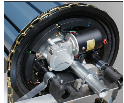
Side View of IGDU drive unit installed on an Industrial Roller Door showing 24 volts DC motors, anti-slip chain guide and chain. Also shown is the anchor block assembly attached to wall bracket with dual anchor pins into the drive housing.
