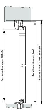
\*\* The structural opening height is based on the finished floor dimension which includes any and all floor coverings. (Please note that each application/project is unique and the tolerance may alter) These doors are rebated on all four sides, failure to take the floor covering into consideration could prevent the door from opening.
