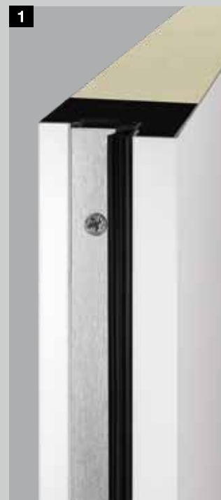
The security door KSI Thermo46 features a 46 mm-thick door leaf and a very good thermal insulation value of up to 1.1 \text{ W}/(\text{m}^2 \cdot \text{K}) .
