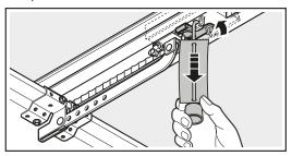
Pull on the cord of the mechanical release.
