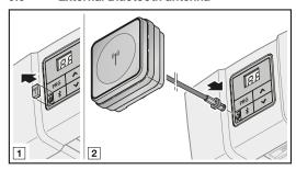
An external antenna is recommended in the event of a limited range.
