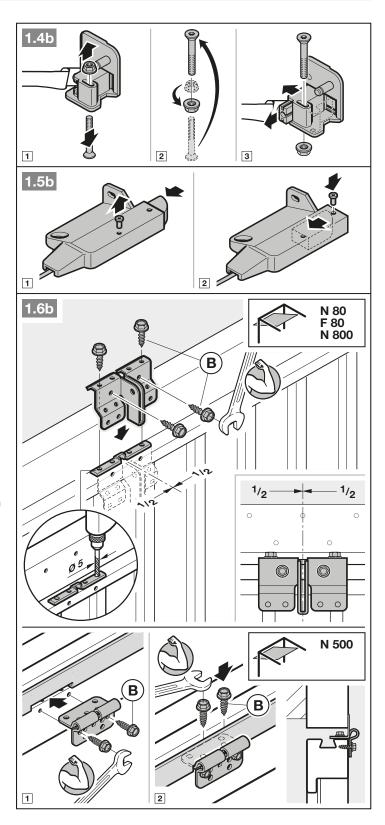
4. In a deviation from the Figures 1.6b/1.7b, the lintel joint and link bracket must be attached off-centre for up-and-over doors with ornamental iron door handles.
