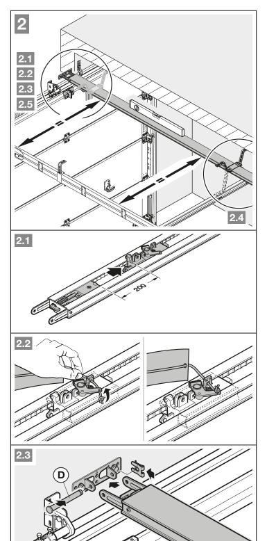
Press the green button and move the slide carriage approx. 200 mm towards the centre of the rail. This is no longer possible once the end stops and operator have been fitted.
