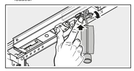
Push the green button on the slide carriage. The slide carriage is re-engaged for automatic operation.
