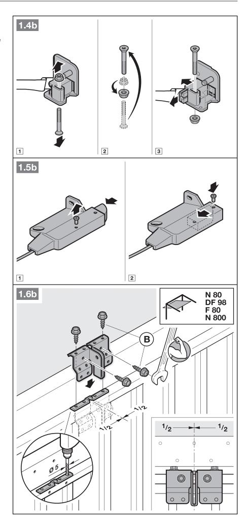
With N80 doors with timber infill, use the bottom holes on the lintel joint for fitting.
