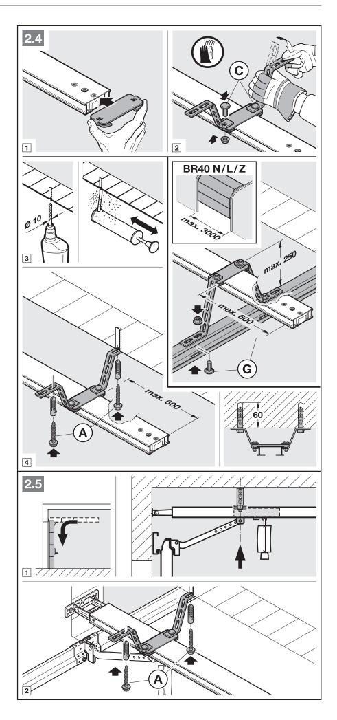
Depending on the **track application**, the installation direction of the fitting bracket must be taken into account.
