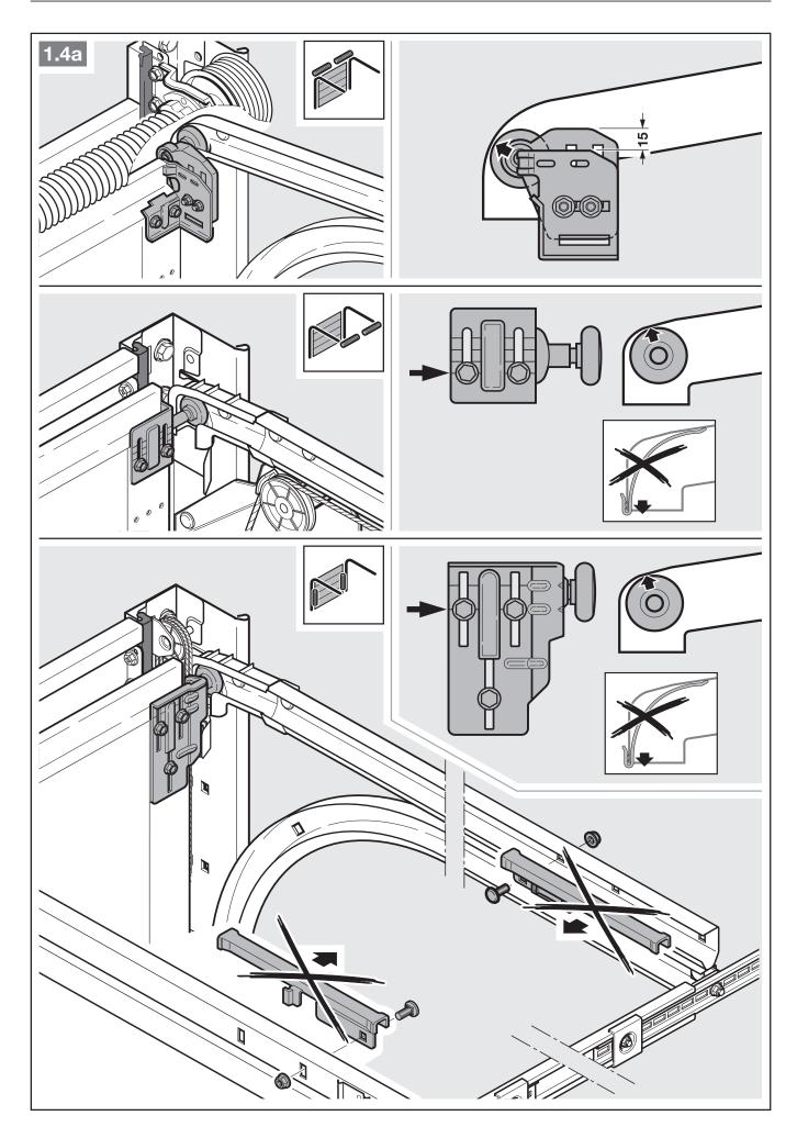
3. For sectional doors with central door locking, fit the lintel joint and link bracket off-centre (max. 500 mm).
