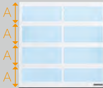
Door version with evenly spaced sections
