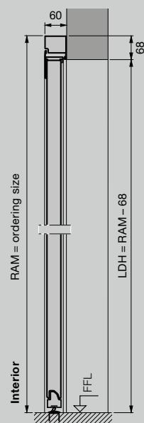
Side door with aluminium block frame, profile type 2
