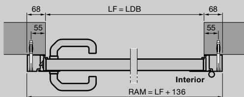
Side door with aluminium block frame, profile type 1
