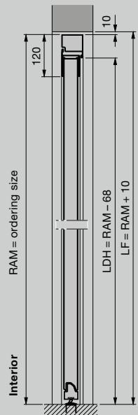
Side door with aluminium block frame, profile type 2
