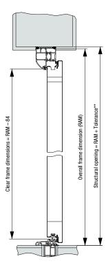
\*\* The structural opening height is based on the finished floor dimension which includes any and all floor coverings. (Please note that each application/project is unique and the tolerance may alter) These doors are rebated on all four sides, failure to take the floor covering into consideration could prevent the door from opening.
