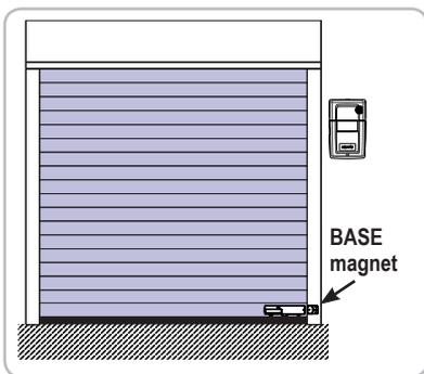
**A base magnet must be fitted for a resistive safety edge.**
