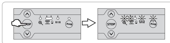
When holiday mode is active, each time a locked control (programming interface or remote control) is pressed, indicator lights 1, 2, 3 and Prog start flashing for 2 seconds.
