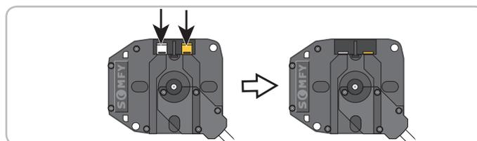
Note: The motor end limits can also be set with a setting tool (ref. 9015971). In this case, set the motor end limits with the cable then move on to step [8] to exit motor adjustment mode.
