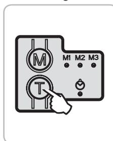
Short press on the T button to activate automatic closure.
