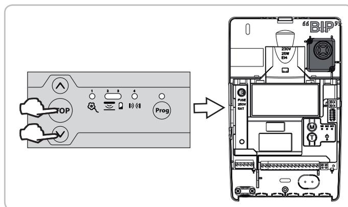
**• Anti-intrusion function test**
