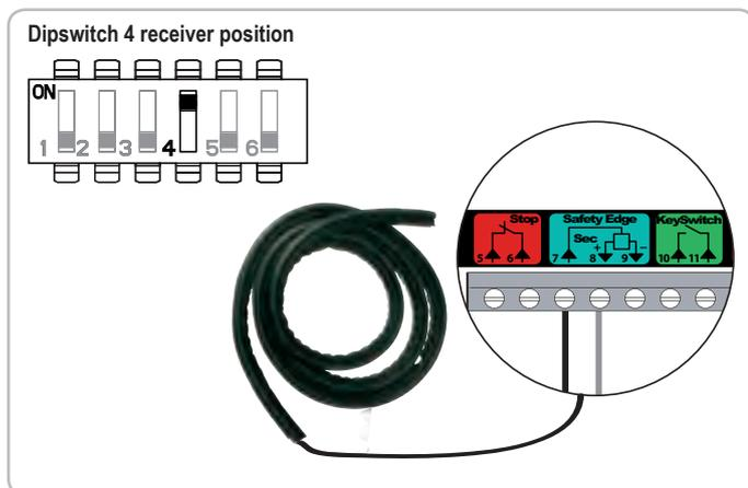
**!** If a wired safety edge replaces a radio safety edge, the radio safety edge transmitter must be cleared (see section 13) to ensure the wired safety edge is taken into account.
