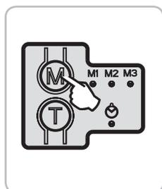
Briefly press the M button to switch from sequential mode to semi-automatic mode.
