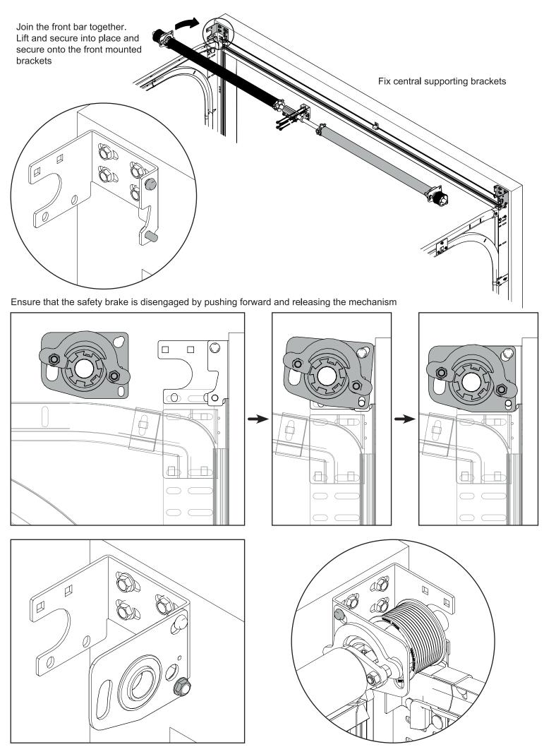
Once the spring mechanism has been fitted, use an M8 nut to secure the components together www.garagedoorsonline.co.uk 01926 463888
