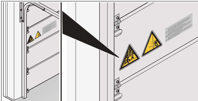
Fig. 1.2 Attach sticker on door panel
