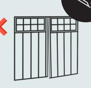
When the frame is set, close the door leaves and check alignment. The top edges of each leaf should be horizontal and level with each other. The door leaves also need to align vertically with the leading edges of each leaf aligned along their full length.
