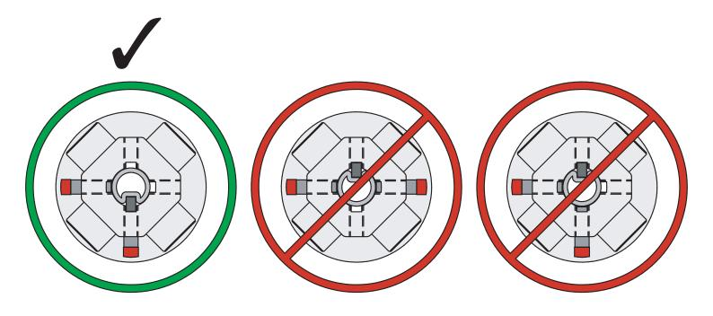
Ensure the locking bolts are pressing down on the key way
