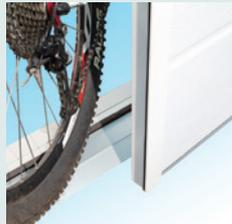
**! A floor that is not level/flat across the full width of the opening will require packing to ensure correct installation of the threshold. If the threshold is not level or distorted, the alignment of the leaves with the seal will be compromised and weather performance degraded.**
