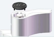
3. Loosen the M6x5 set screw (4mm allen key).
