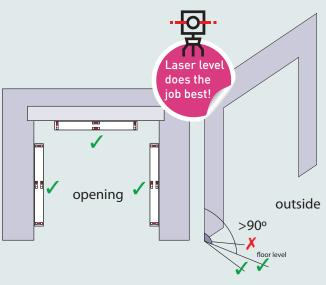
Openings must be plumb and square and the floor area within the arc swept by the door leaf must be level or fall away from the opening.
