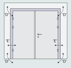
If, after following the above guidance, further alignment is required, use the hinge adjustment to correct the leaf alignment.
