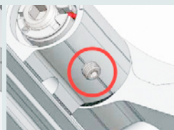
Open the door, loosen the M6x5 set screw
