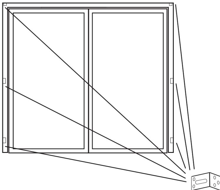
For best results use a laser level. Do not fit to the brickwork as its unlikely to be level and true - **always** fit to your spirit level or laser level.
