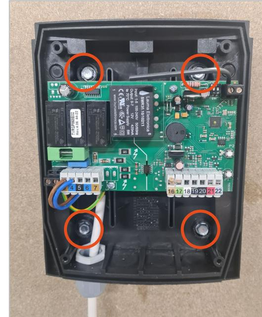
Use appropriate fixings to mount the panel to the structure in the highlighted locations.
