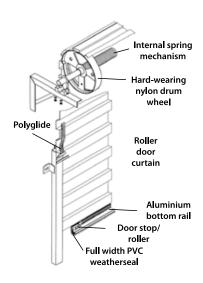
Gildermatic doors require an extra 20mm side clearance on the side the drive unit is required to be fitted.
