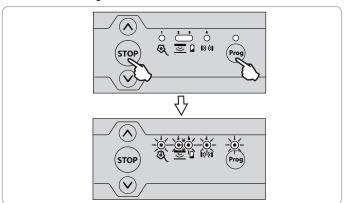
To lock the programming buttons, repeat the locking procedure described above.
