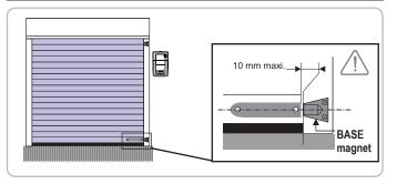
[5]. Press button ⊗ then stop the door by pressing button some to position the garage door in the intermediate position.
