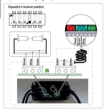
If a wired safety edge replaces a radio safety edge, the radio safety edge transmitter must be cleared (see section 13) to ensure the wired safety edge is taken into account.
