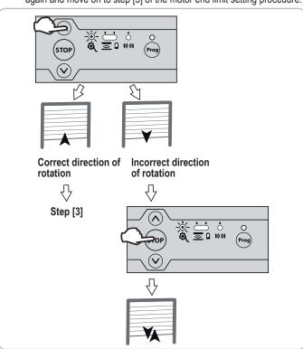
[3]. If the motor end limits are already set, move on to step [8] to exit motor adjustment mode.
